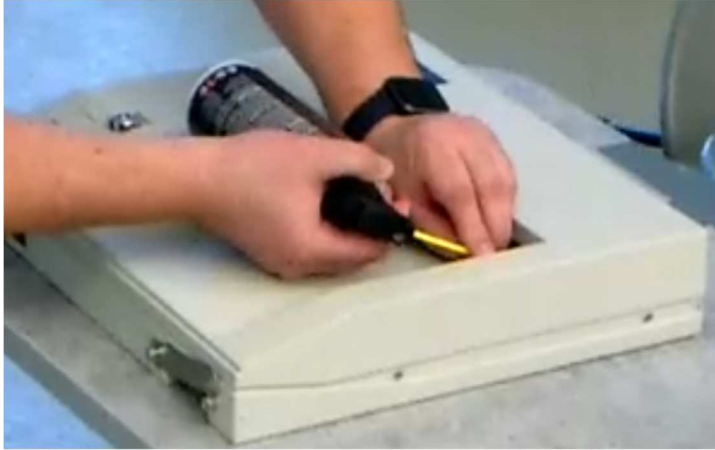
Cleaning the machine with compressed gas [image captured from the livestream]
