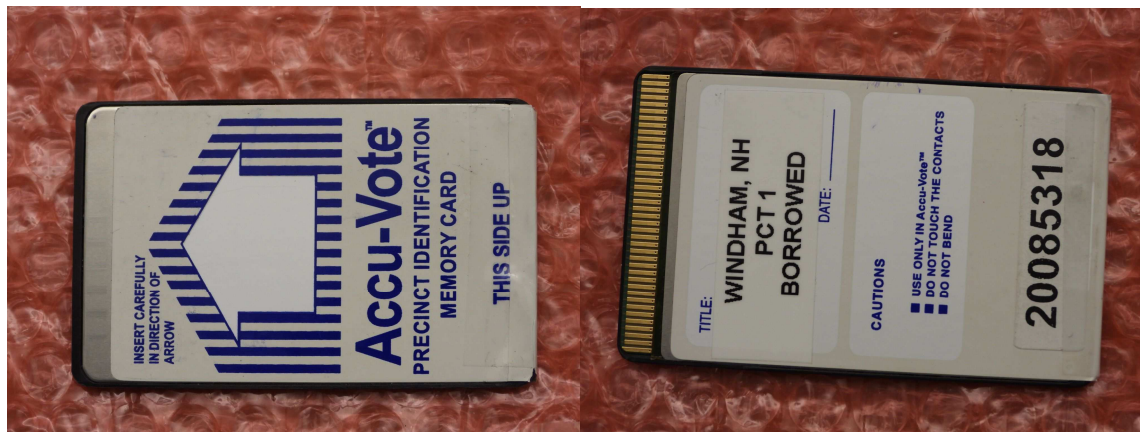
The top and bottom of an AccuVote memory card connecting into a J40 connector
