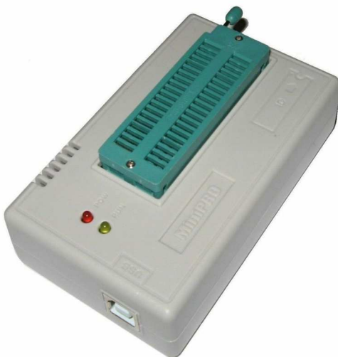
The XGECU device used to read the EPROM chips
