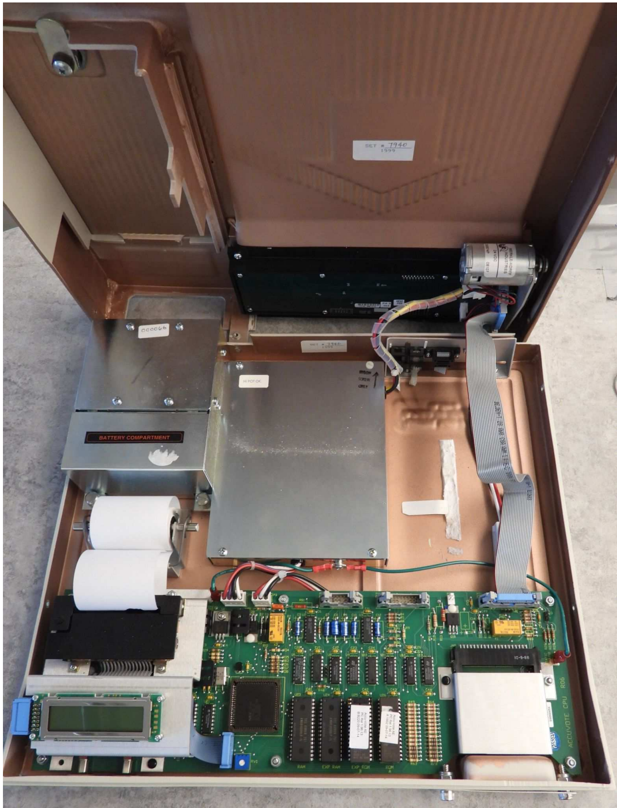
An AccuVote-OS with its cover opened. Notice the line of white powder on the metal box near the center of the picture. (See the discussion of cleaning the scanner beginning on page 96.)
