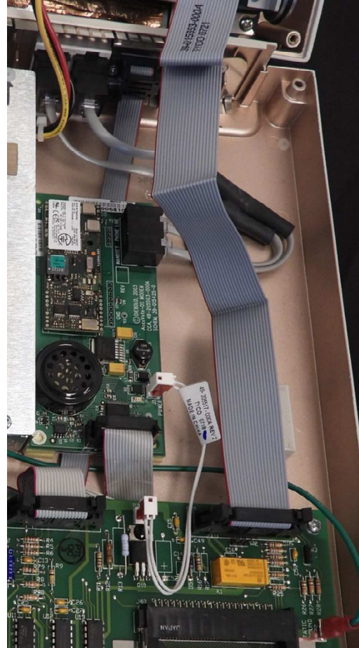
The modem circuit board has been physically removed from the devices used in New Hampshire
