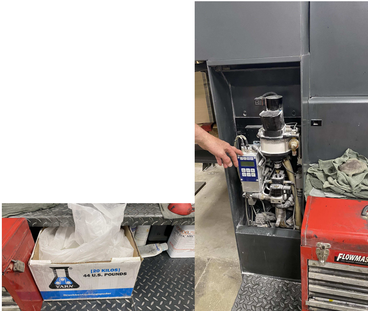
Application of Varn anti-set-off (offset) powder 62
